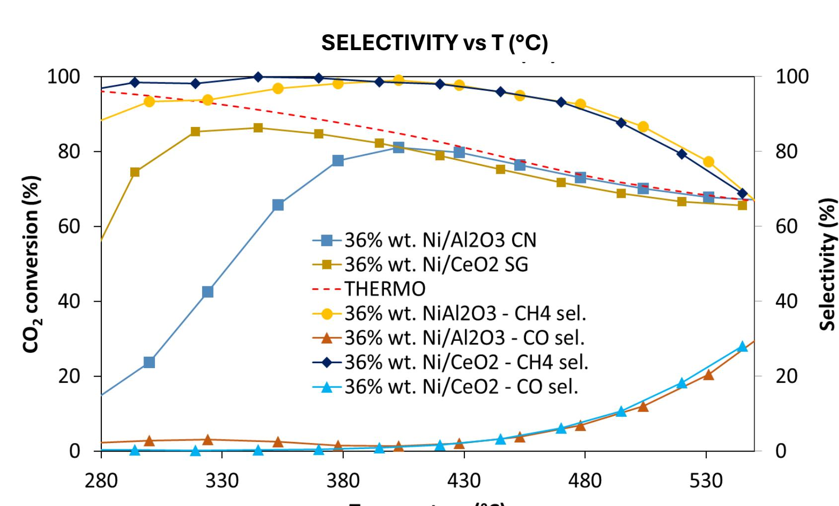
$\text{CeO}_2$  supported catalyst approached the thermodynamic  $\text{CO}_2$  conversion (86%) with complete selectivity towards  $\text{CH}_4$  at 345°C
