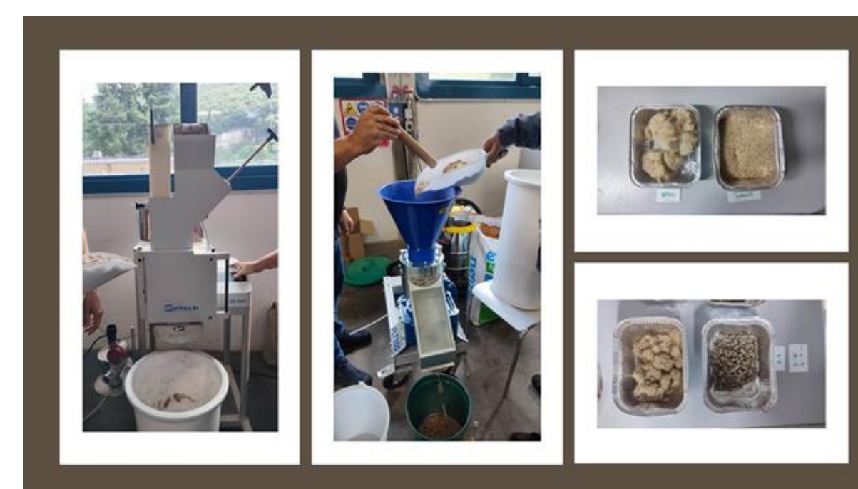
Figure 1. Cutting mill on the left and pellet machine at the center. On the right the matrices wool and sawdust. On the bottom right, an example of mixture (11) and pellets (11)
