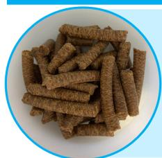
As feedstock we have selected **different residual press-cakes** from mechanical extraction of various oleaginous seeds.
