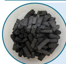
**Slow pyrolysis** was chosen as reference technology because it allows to maximize the biochar production.
