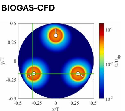
Example non-OŤ the dimensional velocity in an horizontal cross-section of a CFD digester. allows to identify dead zones and shear critical stress conditions.
